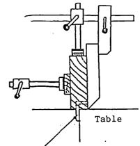
Edge of planer knife must clear end of block and outfeed table edge
