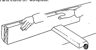
When edging a workpiece of more than 75mm thickness, move the piece forward with both hands. In doing so, the left hand, fist closed, presses the workpiece against the fence and the outfeed table. The right hand lies upon the workpiece.
