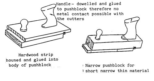
Abrasive paper glued to base to give better frictional grip and prevent the workpiece moving sideway
