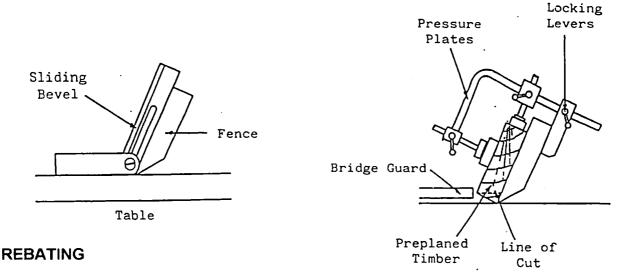
Provided that it is not a stopped rebate, this operation can be done on the *Sedgwick* planer range provided it is effectively guarded. The Shaw Guards must be used to ensure this operation can be done safely.
