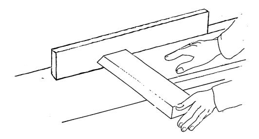
The work should be fed by the right hand, and if the knives are sharp and the tables are properly set the main functions of the left hand are to assist feeding by drawing the wood along the delivery table towards the end of the cut, and to remove the planed piece.
