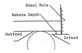
The size of rebate will determine whether or not it can be done at one pass. Two or more cuts may be required, but it must be remembered that the maximum depth of cut is 16mm, and rebates in excess of this will have to be done on other machines. Ensure that the shaw guards are positioned as shown over the page.
