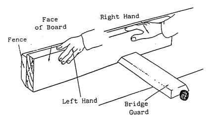
When flatting a workpiece of more than 75mm thickness the bridge guard must be lowered on to the table and adjusted horizontally to the workpiece. The workpiece should be straightened, with flat hands beside the guard, along the fence.
