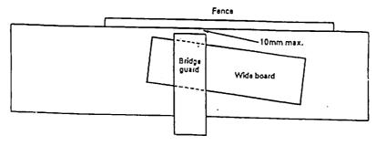
As it is illegal to operate the surface planer without the bridge guard, the long accepted way of placing the front portion of timber on the outfeed table and taking several cuts off the other end then reversing the timber should not be used.
