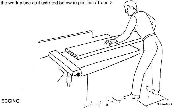
When edging, the wood is passed between the end of the bridge guard and the fence. The bridge guard should be adjusted both horizontally and vertically to leave only 10mm from both the feed table and the workpiece, as shown below:
