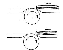
Working round side down causes timber to rock, thus making it very difficult to obtain a straight parallel face.
